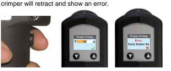
The cycle button must be held down until the crimp is complete. If the switch is released early the
